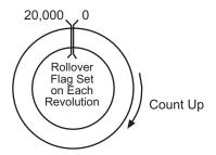
The above figure illustrates counting in a clockwise direction.
