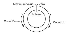
Sample Configuration Simple Ring Counter w/ Flags (20k Limit):
