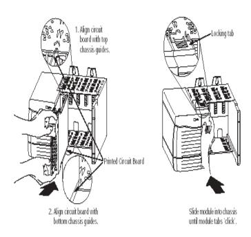
2. Slide your module into the chassis until both top and bottom retaining clips are secure. Apply firm even pressure on your module to attach it to its backplane connector. Never force your module into the slot.
